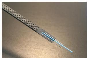
**T**he FN-SILL-3 is designed for strain and temperature measurements. It consist of 2 optical fibers (in the cable center) and 2 reinforcing bars, which allow cable to sustain up to 25 kg force.
