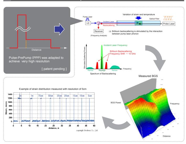
Neubrex technology of PPP-BOTDA successfully increases the spatial resolution and strain accuracy one-order higher than previous products. This is the only one technology in the world.
