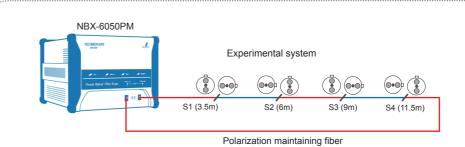
Measure manually by switching polarization of 0° and 90°  $\,$
