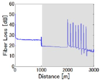
The OTDR offers the measurement of trunk and reflection peaks of branch paths.
